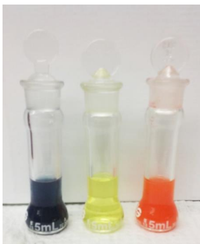
Fig. 6. Individual color additive molecule experimental batches prepared in ethanol solvent.
