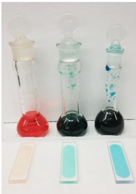
Fig. G2. Heterodimeric mixtures of individual color additives in ethanol solvent. From left to right: FD&C Yellow No. 5 and FD&C Red No. 40 (Tartrazine—Allura Red), FD&C Yellow No. 5 and FD&C Blue No. 1 (Tartrazine—Acid Blue 9), and FD&C Blue No. 1 and FD&C Red No. 40 (Acid Blue 9—Allura Red) in ethanol solvent.
